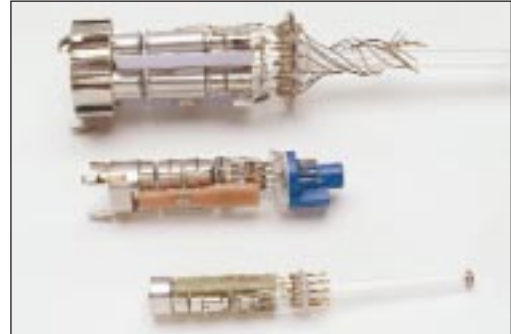
Fig. 1 - Today's electronic guns have gotten smaller and are capable of producing better quality pictures.
